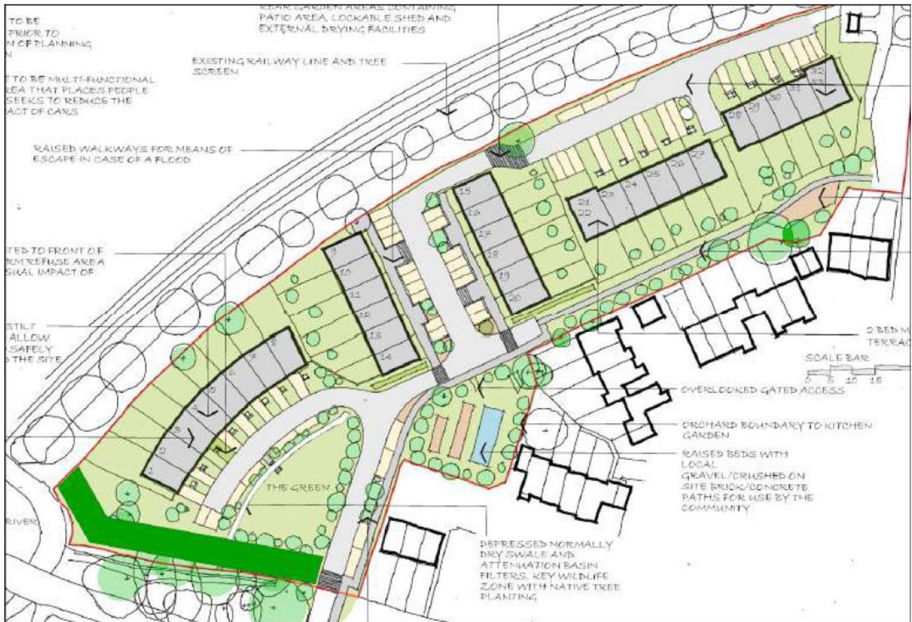
12/P/01005 Swale Option 1: 1m deep | 6.5m wide | 64m total length
