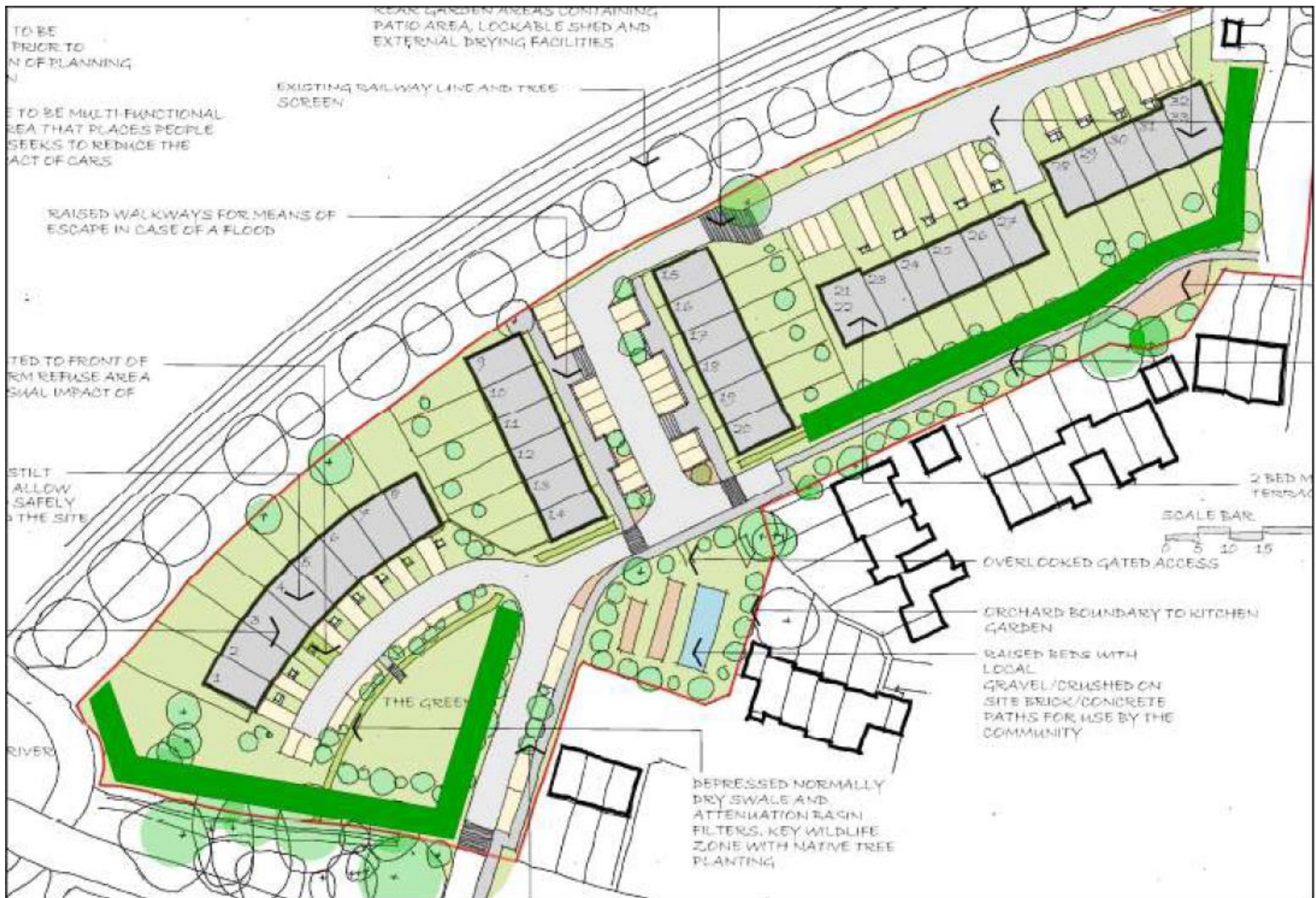
12/P/01005 Swale Option 2: 0.6m deep | 4.1m wide | 200m total length
